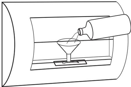
Using the funnel provided or your own funnel, carefully pour in the liquid ethanol fuel for fireplaces into the reservoir until it can be seen above the perforated holes in the reservoir. If any fuel does spill, you should always wipe it up prior to lighting your fireplace.
