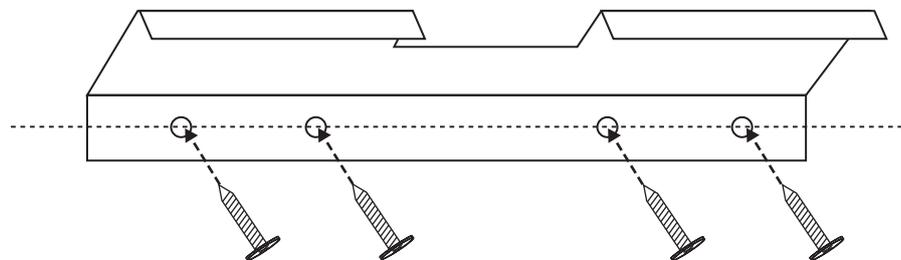
Place bracket over holes of anchors and attach to the wall by inserting anchor screw through the bracket into the anchors in the wall. Repeat for all four screws.
