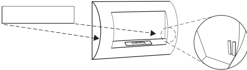
Insert glass panel into the slots located on the inner sides of the fireplace.
