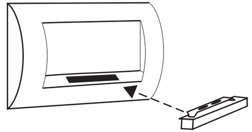
Insert fuel reservoir into fireplace and cover fuel reservoir with the provided lid.
