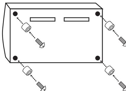
Using a screwdriver, attach wall spacers to the back of the fireplace in the predrilled holes using the spacer screw. If they are already attached, insure it is on securely.
