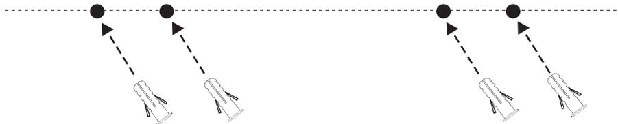
Insert the wall anchors flush into holes in wall as shown in step 3. A light tap with a hammer might be necessary to insure it is inserted flush with the wall. If you drill a hole into a wooden stud, the wall anchor is not necessary.
