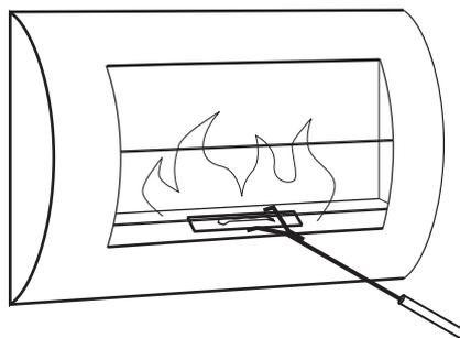
The curved ends in the handle provided will fit into the holes in the lid of the reservoir. You can adjust the flame height to get the desired flame height, heat output, and length of time fuel lasts. When you are ready to extinguish the fireplace, use the handle to slide the lid of the burner completely closed over the opening to cut off the oxygen supply to the fuel. This will snuff out the flame. It may take a few seconds to completely extinguish the flame.
