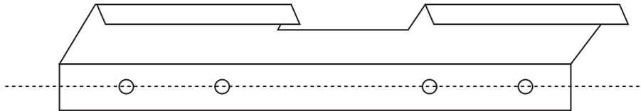
Use a level to mark a straight line with a pencil on the wall where you will mount the bracket. The wall should be made from drywall, tile, brick, stone, ect. It must not be flammable (e.g. no wallpaper or wood) Make sure you mount the fireplace at least 4 feet away from any drapes or flammable materials.
