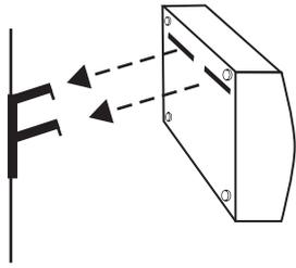
Hang fireplace on the wall by placing the open slots on the back of the fireplace onto the mounted bracket.
